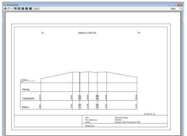
Creation details: Many scales for heights and distances, many paper formats, 0 - 3 decimal places for heights and distances, raising the profile base, reduction of distances to any point of profile, addition of a start distance (e.g. for longitudinal profiles), variable text for the lines *Planning, Topography and Distance*, calculation of profile areas. In addition to the topographic profile it is also possible to create profiles from planning heights.
